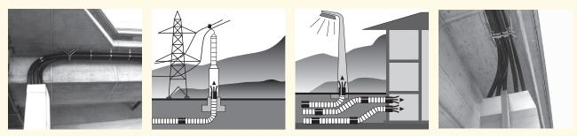
• outer protection of electrical lines and cables • utilization with offset bends, goosenecks, S-shapes, T-sections and other connecting options
