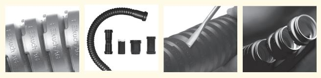
· pioneering cable protection made of durable synthetics · no material loss · segment components can be lengthened or shortened as desired • the endless connecting system can be three-dimensionally bent and curved with a choice of angle • merely one simple tool, a screwdriver, is necessary to open the pipe
